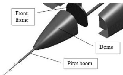
Figure 6. Pitot boom location on the vehicle.
