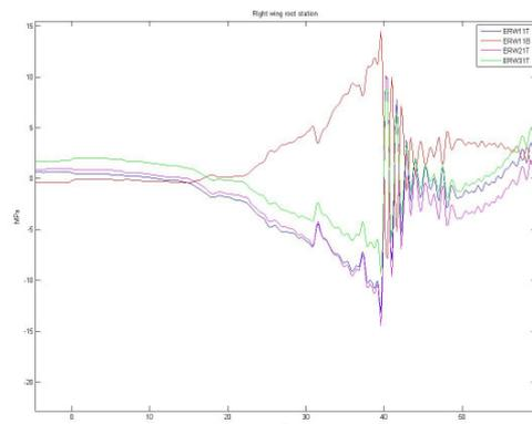
Figure 17. Stresses on caps of right wing root section.
