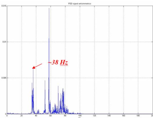
Figure 19. 1<sup>st</sup> anti-symmetrical bending frequency of wing.
