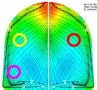
Figure 15. Base plate with the sensors location
