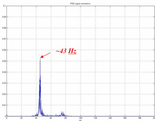
Figure 18. 1<sup>st</sup> symmetrical bending frequency of wing.
