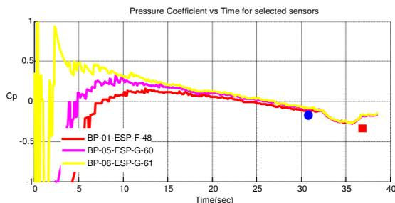
Figure 16. Measured base Cp compared predictions
