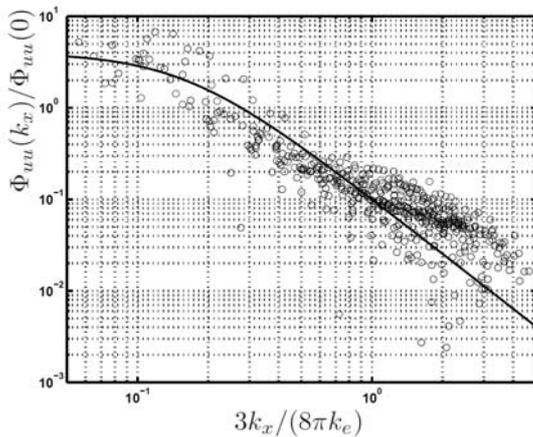
Figure 7 – Normalized axial turbulence spectrum extracted from CFD computation (o) and von Karman turbulence model (plain).
