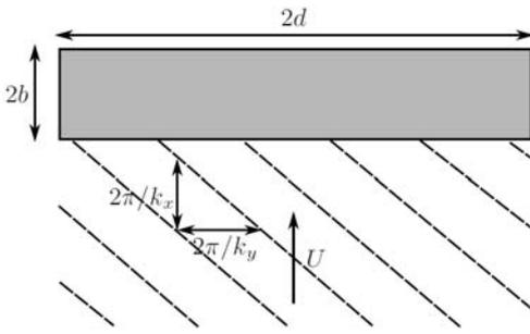
Figure 3 – Representation of a single skewed gust incident the airfoil
