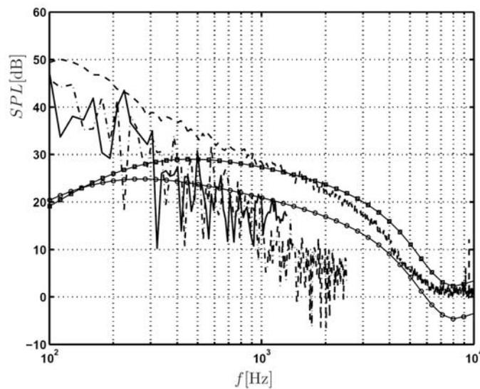
Figure 9 – SPL for an airfoil in a turbulent jet at a listener placed at  $\theta = 90$  deg and  $r = 0.3$  m obtained with experiments (dash), CFD Case 1 (dash-dots), CFD Case 2 (plain), and predicted with the Amiet's theory for a 2D span airfoil and  $U = 0.49U_0$  (plain-square) and for a 1D span and  $U = 0.8U_0$  (plain-circle).
