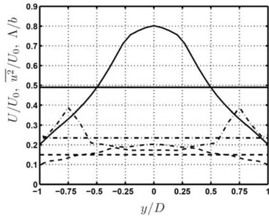
Figure 8 – Normalized mean velocity (plain), turbulence intensity (dash) and normalized turbulence scale (dash-dot) along the airfoil span and their mean value in the range  $y \in [-1, 1]$ .
