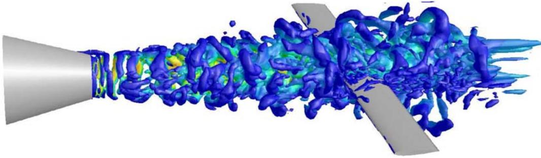
Figure 5 – Instantaneous flow field around the airfoil, coherent structures visualized with the second invariant of the velocity gradient tensor  $Q = 30000$  colored by dynamic pressure.
