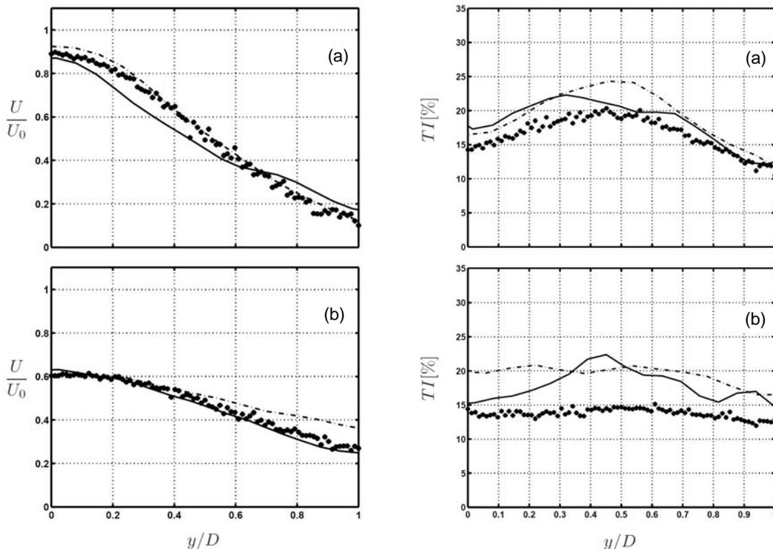
Figure 6 – Mean velocity profiles and turbulence intensity profiles, experimental (symbols) and numerical case 1 (dash-dot) and case 2 (plain), for  $y = 5D$  (a) and  $y = 8D$  (b).
