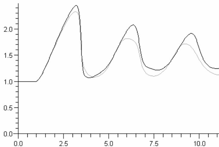
Figure 3. Mach number profile along the free jet axis ( $N=2$ ). Calculated (dark) and measured (gray) results.
