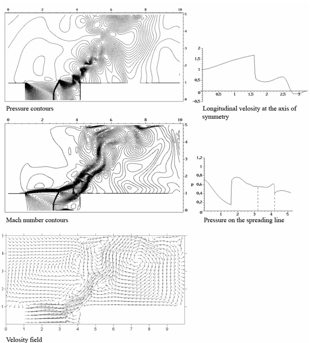
Figure 9. Snapshot of the jet/barrier interaction at  $t = 124.76$
