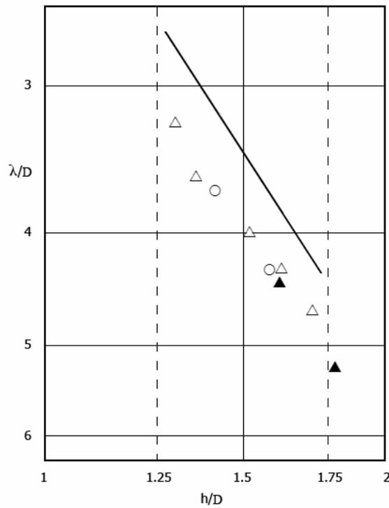
Figure 6. Comparison of the calculated and measured data on the frequency (wavelength) of the sonic underexpanded impinging jet fluctuations ( $N = 2$ ). — Calculation,  $d = D/D_a = 1$ ;  $\triangle$  [7],  $d = 1$ ;  $\blacktriangle$  [9],  $d = 0.58$ ;  $\circ$  [10],  $d = 1.1$
