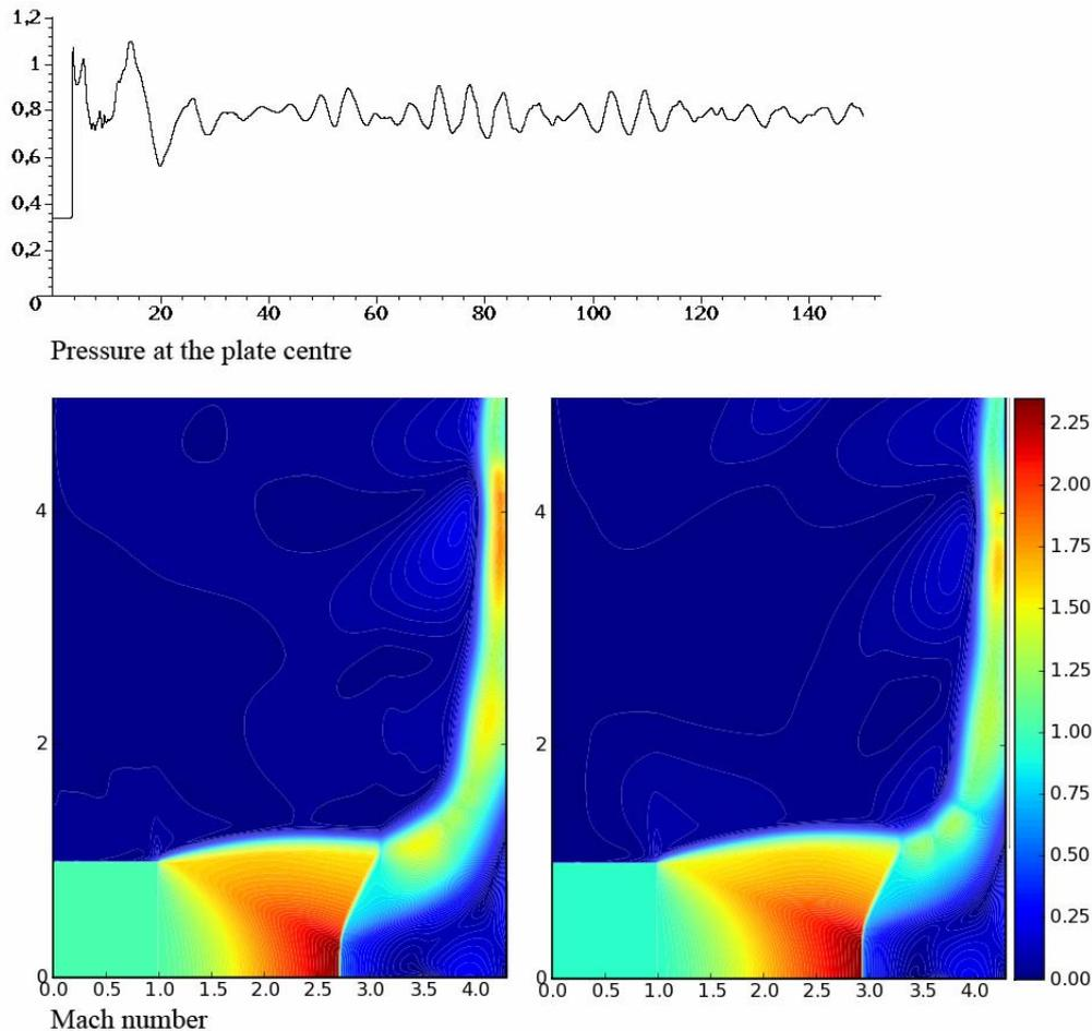
Figure 13. Impingement of the sonic jet on an infinite plate ( $N = 2$ ,  $L = 3.3$ )
