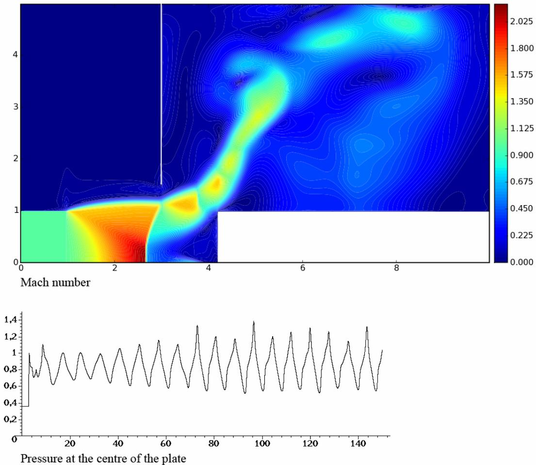
Figure 12. Self-oscillations in the presence of an annular screen in the external acoustic field ( $N=2$ ,  $L=3.2$ )
