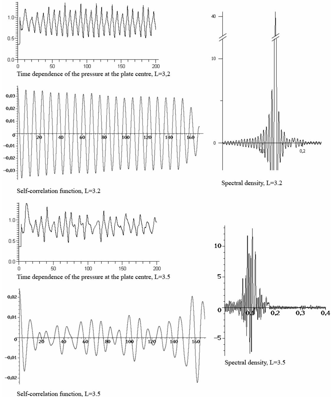
Figure 5. Spectral characteristics of self-oscillation process for  $N = 2$ ,  $L = 3.2$  and  $L = 3.5$
