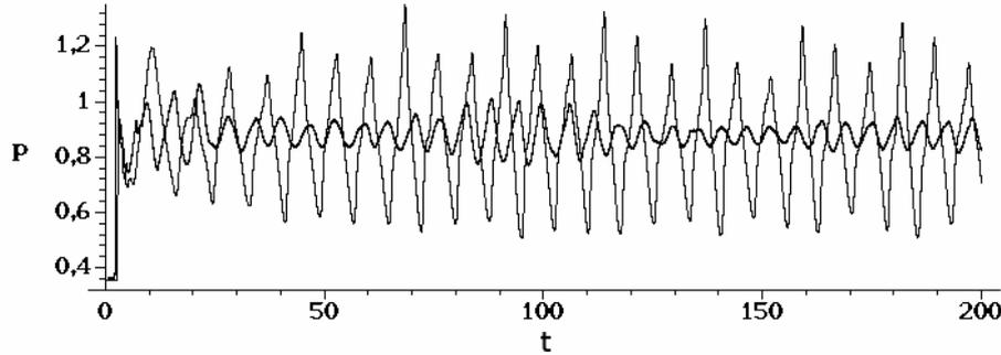
Figure 4. Time dependence of the pressure at the centre of the plate for  $N = 2$ ,  $L = 2.7$  and  $L = 3.2$
