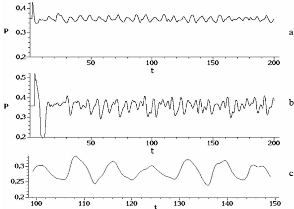
Figure 11. Acoustic disturbances in the external field [ $x = 1, y = 2.5$  (a) and  $x = 4.2, y = 2.5$  (b)] and inside the jet [ $x = 2.4, y = 0.8$  (c)]  $N = 1, L = 3.2$
