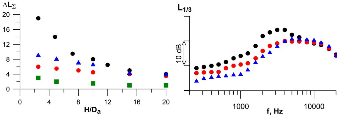
Figure 1. The influence of jet deflector shape on overall sound pressure level and 1/3-octave sound pressure spectrum ( $M_a = 3,5$ ;  $n = 1,0$ ;  $T_o = 300K$ )
