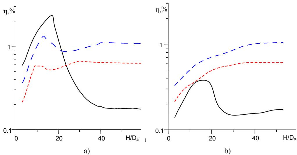
Figure 6. Acoustic efficiency of the system "jet-deflector" ( $M_a=3.0$ )
