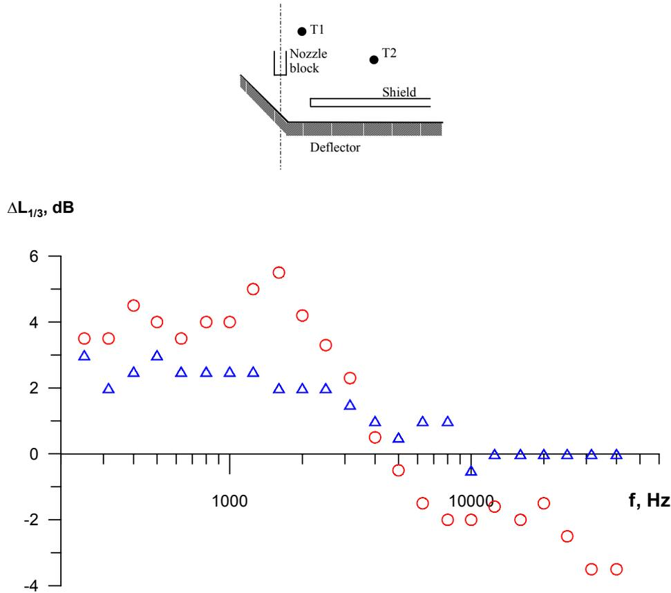
Figure 5. Dependency  $\Delta L_{1/3}$  against jet acoustic radiation frequency  $f$  ( $\circ$  – in point T1,  $\Delta$ - in point T2);  $M_a = 3,2$ ;  $n = 1,0$ ;  $T_o = 2200K$ ;  $H/D_a = 4,0$
