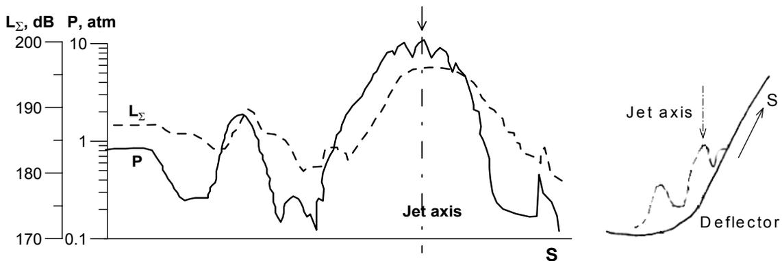
Figure 2. Typical distributions of static pressure  $P$  and rms levels of pressure fluctuations  $L_{\Sigma}$  along generatrix of single slope deflector surface ( $M_a = 3,0$ ;  $n = 0,9$ ;  $T_o = 300K$ ,  $H/D_a = 6,3$ )
