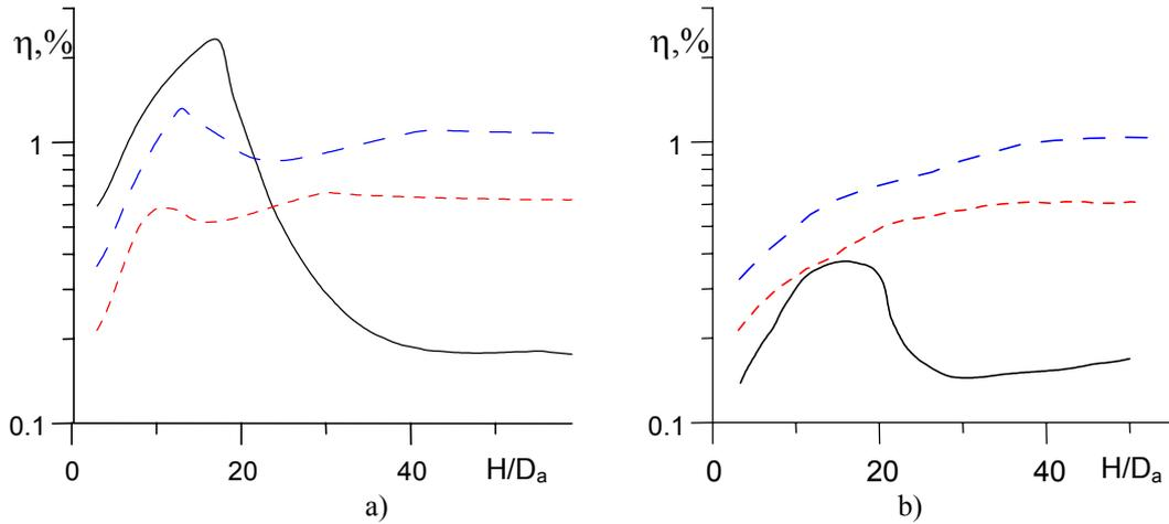
Figure 7. Input of different regions of noise generation ( $T_o = 2500K$ ;  $\gamma = 1.25$ ;  $M_a = 3.0$ )
