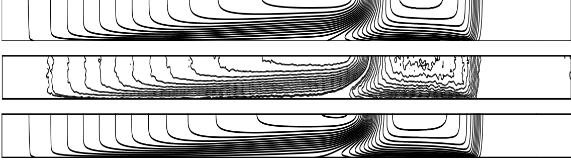
Figure 1: Temperature flowfields at Kn_1 = 0.05 obtained in Navier-Stokes (top), DSMC (middle) and BGK (bottom) simulations.
