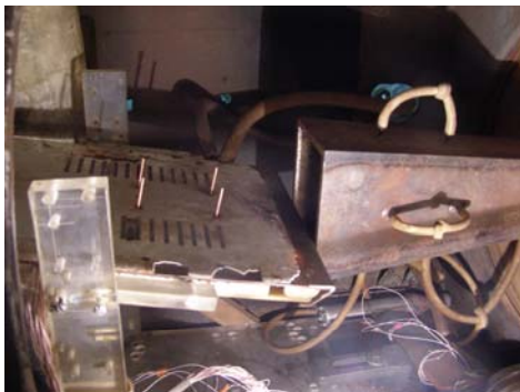
Fig. 27. Model in the test section with Smaller Nozzle before test
