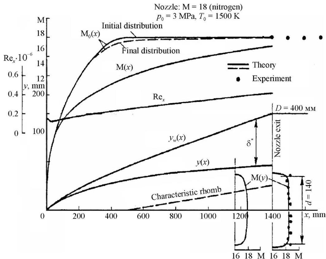
Figure 4. Comparison of theoretical and experimental flows in nozzle at  $M_p = 18$
