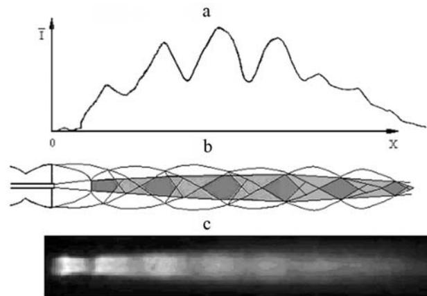
Figure 2. Hydrogen combustion unevenness in supersonic nonisobaric air jet. *a* – integral radiation intensity of the H<sub>2</sub> flame in the axial direction; *b* – scheme of gasdynamic structure with combustion zones of various intensity; *c* – 2-D distribution of radiation intensity in ultraviolet range.
