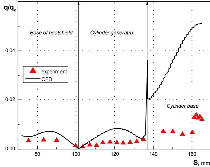
Figure 6. Relative heat flux distribution in the base region. IT-2. Nitrogen flow.  $M_\infty=20.4$
