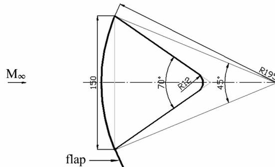
Figure 8. Model of Martian descent vehicle (MDV)
