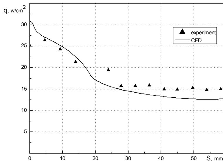
Figure 4. Heat flux distribution along heatshield surface. IT-2. Nitrogen flow.  $M_\infty=20.4$
