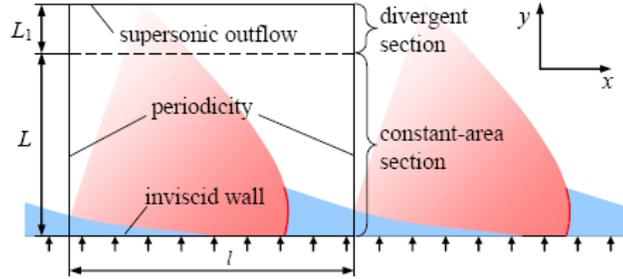
Fig.2. Computational domain for CDWE simulation
