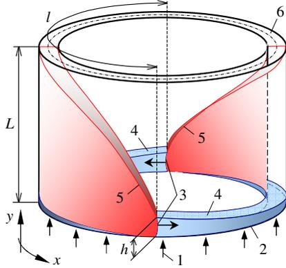
Fig.1. Schematic of CDWE combustion chamber.
