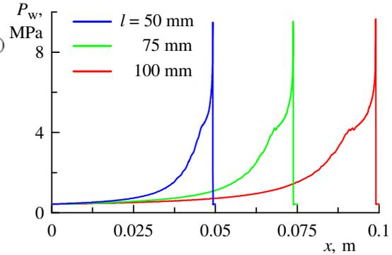
Fig. 9. Instantaneous distributions of wall pressure for different azimuthal periods.
