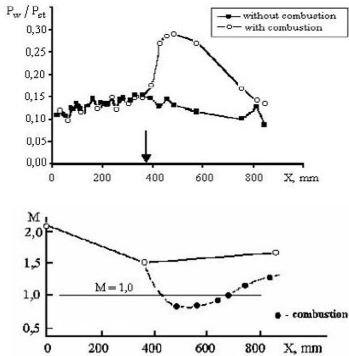
Figure 3.  $M=2$ ;  $T_1^0=1850$  K; mixture of 50%  $H_2$  + 50%  $C_2H_4$ .
