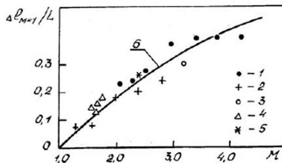
Figure 4. The length of the supersonic interval of the pseudoshock:
