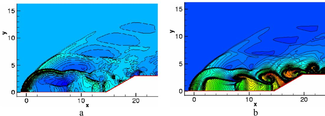
Figure 4. a) Contour of pressure, b) contour of Mach number
