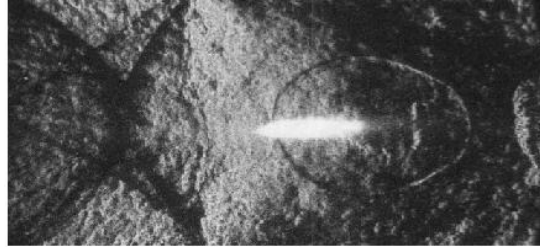
Figure1. Optical discharge in supersonic flow (M=2.0, d=20mm, f=50 kHz)
