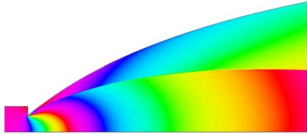
Figure 7. Flow in the nozzle with abrupt diversion when nonoptimal contour of its supersonic part
