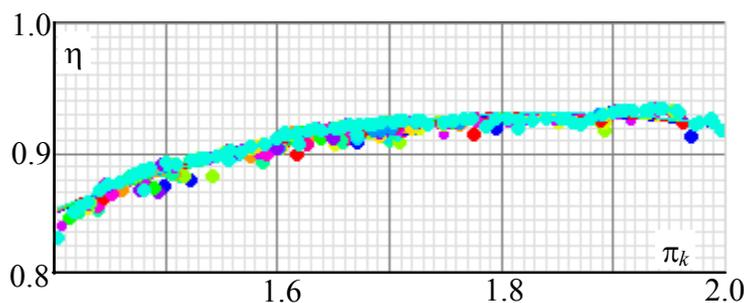
Figure 11. The Pareto-front when optimization of fan's blade
