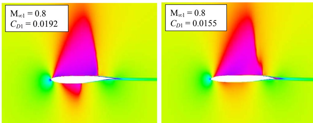
Figure 9. Flow of airfoils, designed by method <sup>27</sup> (on the left) and
