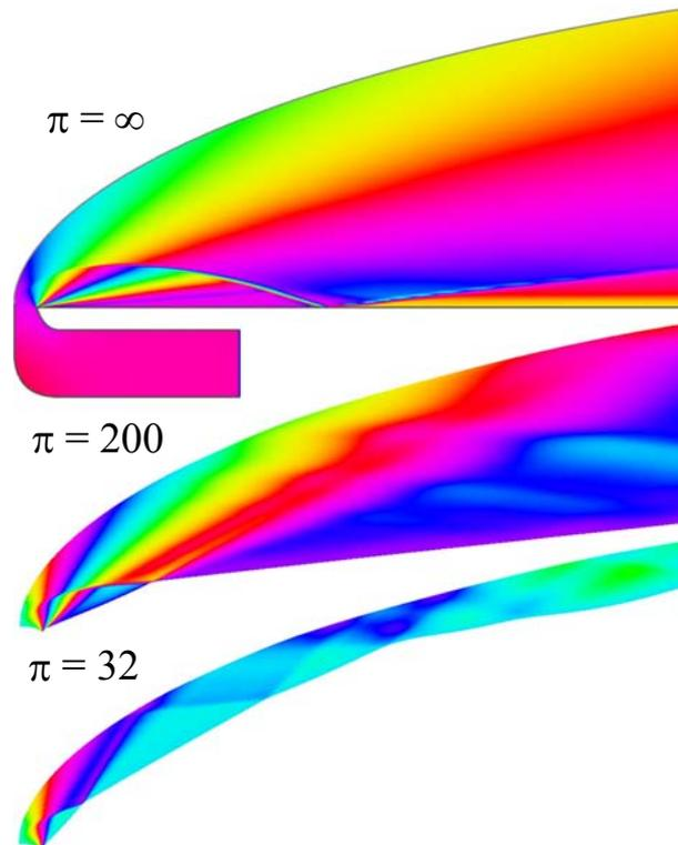
Figure 6. Flow in optimal expansion-deflection nozzle when design and on-design conditions
