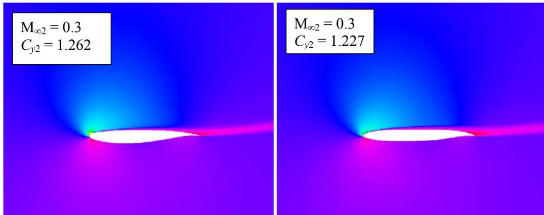
Figure 10. Flow of airfoils, designed by method <sup>27</sup> (on the left) and by GA (on the right) when  $M_{\infty 1} = 0.3$
