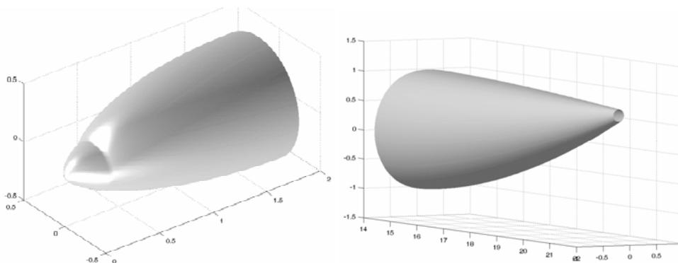
Figure 2. Shapes for the nose and tail sections surfaces
