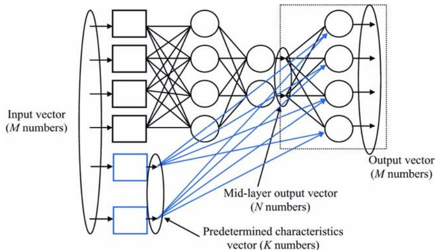
Figure 8. RANN modification. Generation of objects with predetermined characteristics
