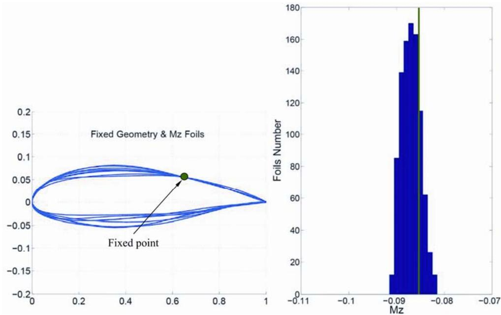
Figure 9. Set of airfoils with initially imposed limitations on geometry and aerodynamic characteristics. Geometry and  $m_{z0}$  distributions over the airfoils.
