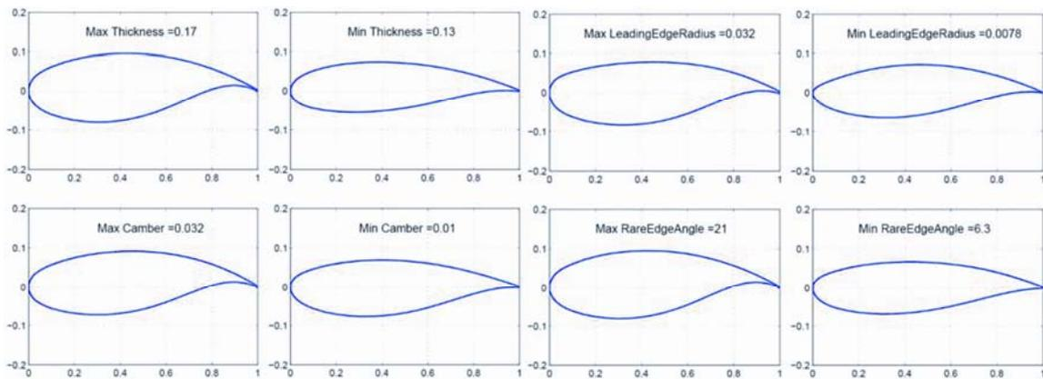
Figure 7. Random generation of airfoils within the 6D space
