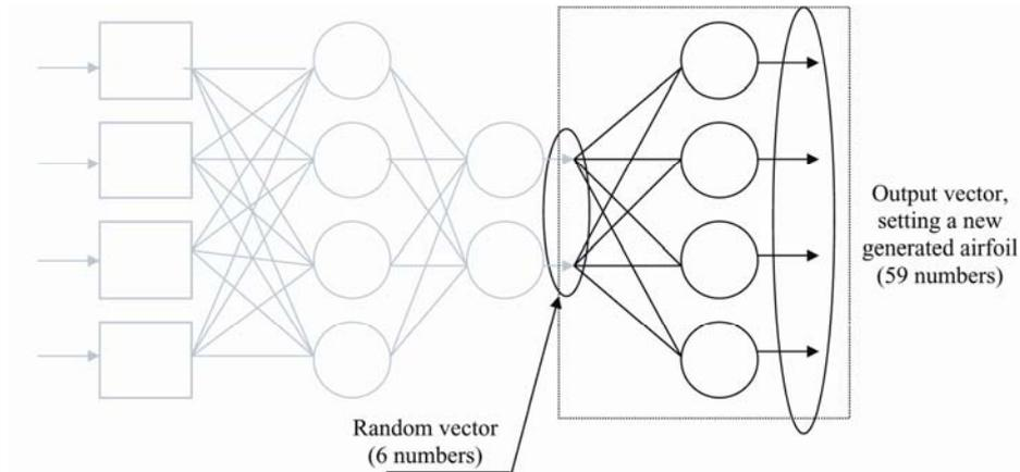
Figure 6. Airfoil generator: deriving airfoil geometry from a random vector of the compressed data space
