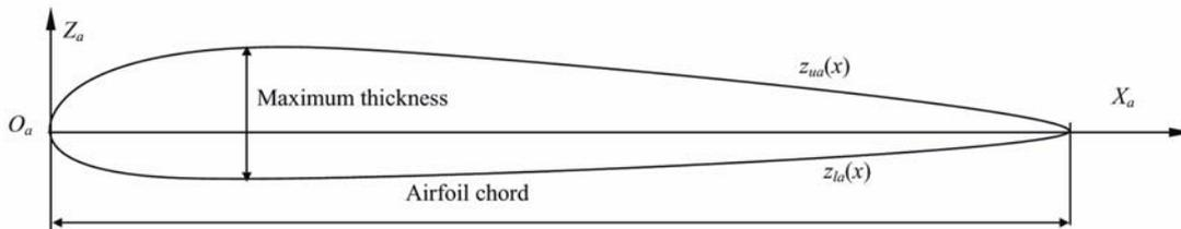
Figure 4 – Airfoil coordinate system
