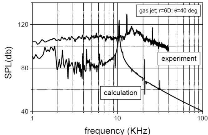
Fig. 10. Comparison spectral characteristics of sound obtained by computation and experiment.
