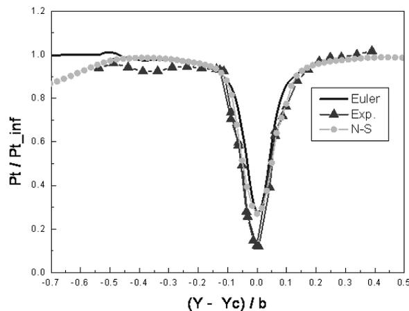
Fig. 4. Pitot pressure distributions through the vortex core.
