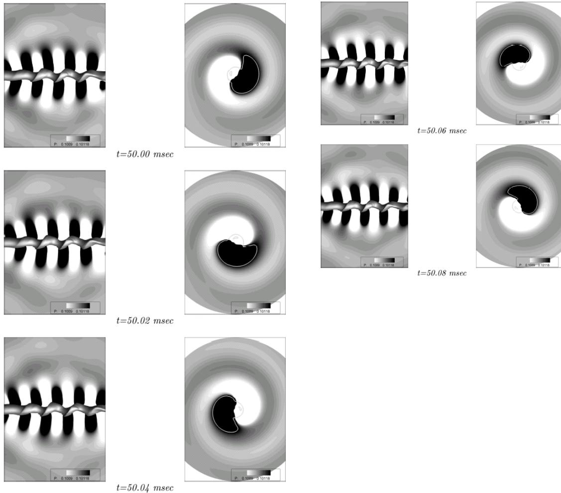
Fig. 7. Jet boundary ( $\rho=1.7 \text{ kg/m}^3$ ) and pressure in the ambient gas: meridional plane (left), cross-sectional plane  $x=13D$  (right).
