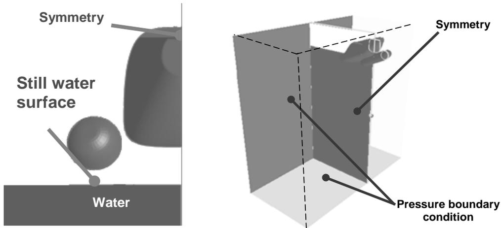
Figure 6. CFD model of helicopter splashdown.
