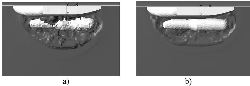
Figure 11. Comparison of water distribution over the helicopter for a) soft and b) rigid ballonets, time is 0.825 s after splashdown.
