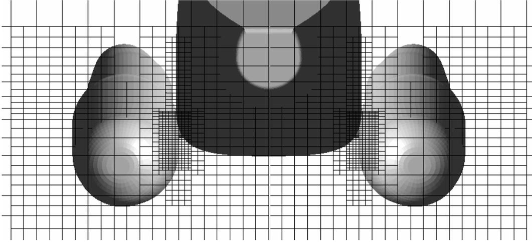
Figure 3 CFD mesh with Local Adaptation and Sub-Grid geometry resolution
