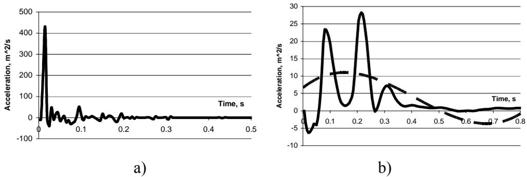
Figure 9. Vertical acceleration of helicopter center mass.
