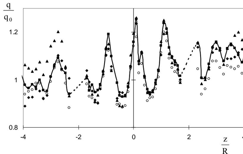
Fig.2 Heat flux distribution along the cylinder leading line<sup>7</sup>. Wind tunnel tests at  $M_\infty=6.1$ ,  $Re_\infty \approx 1.7 \cdot 10^5$ .
