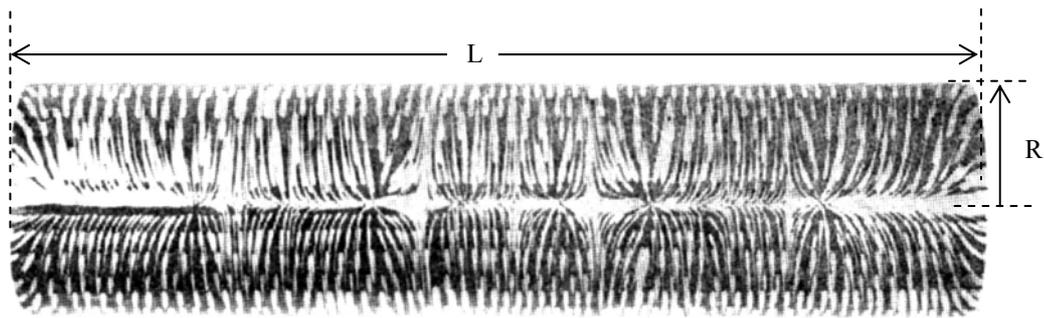
a)  $M=3$  ,  $L/R=8$  ,  $Re=3 \times 10^6$
