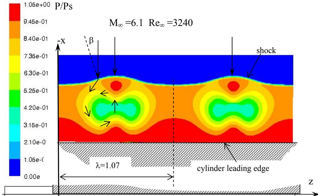
Fig.5. Scheme of calculation domain and pressure field  $P/P_s$  on the symmetry plane  $y=0$  at  $M_\infty=6.1$ ,  $Re_\infty=3240$ ,  $Re=2700$ ,  $\gamma=1.4$
